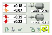
Rotate the sensors to the third position and measure. The results will be displayed on screen. Press the shim icon.
