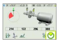
Rotate the sensors to the second position. Press the measurement icon again to take the second measurement.
