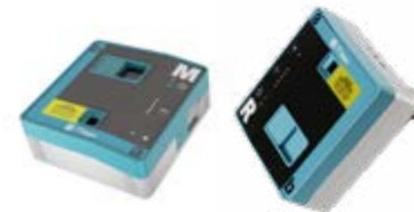
MEAX SR201 and SM201 serve as multifunctional sensors. They both have an integrated laser transmitter, a 2-axis PSD detector and a high-resolution inclinometer to record the angle of rotation. The sensors are used for a variety of types of measurements such as straightness, squareness, spindle direction, and coaxiality. The SR unit (marked R) is fitted to the part of the machine which forms a reference, and the SM sensor (marked M) is fitted to the machine axis that is to be measured.
